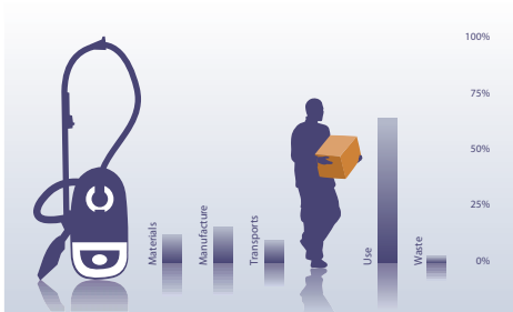
Figure 2. Result from an LCA study for a vacuum cleaner and the relative importance of the different life cycle stages in the total environmental impact (Source: EPD Vacuum cleaner, ETA, www.environdec.com )
