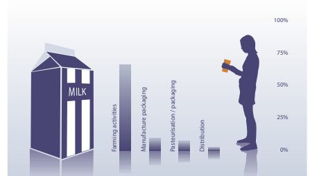
Figure 3. Result of an LCA study of 1 litre of packaged milk and the relative importance of the different life cycle phases in the total environmental impact (Source: Climate declaration Bottled Milk, Granalo, www.environdec.com )
